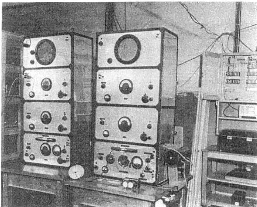
Two Multivibrators working off clocks. Note stop-clock in foreground. Also very neat double dial stop watch. Loud speakers to note beats at top.
