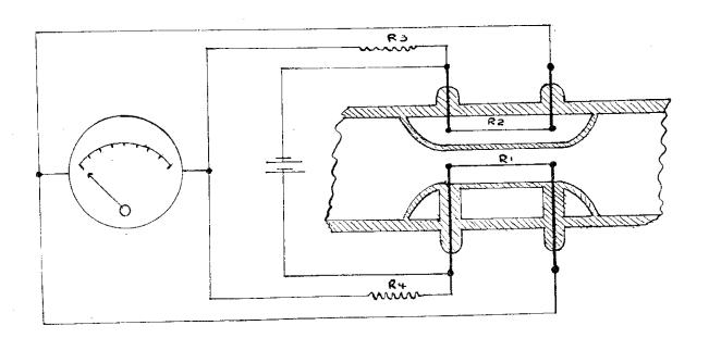
The action of course is that the cooling effect on R<sub>1</sub> will be a function of the velocity of the gas flowing through the narrow tube. Measurements of small changes in pressure are obtained by sealing the tube into a large hollow sphere, all other details as above. Any change in atmospheric pressure will cause a flow into or out of the sphere and so affect R<sub>1</sub>.
