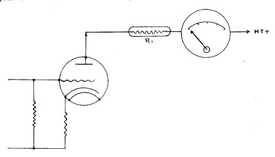
Any increase in anode current brought about variation of grid volts will raise the temperature of R1 thereby lowering its resistance and bringing about a larger increase in anode current per unit change in grid volts than would have otherwise been the case.
