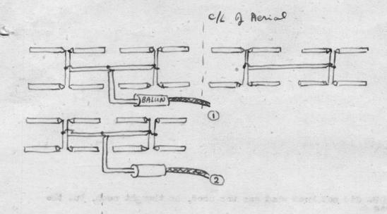
elements and careful impedance transformation, together with the matched phasing lines, has resulted in a system which requires no adjustment over the range 119 - 156 Mc/s.
