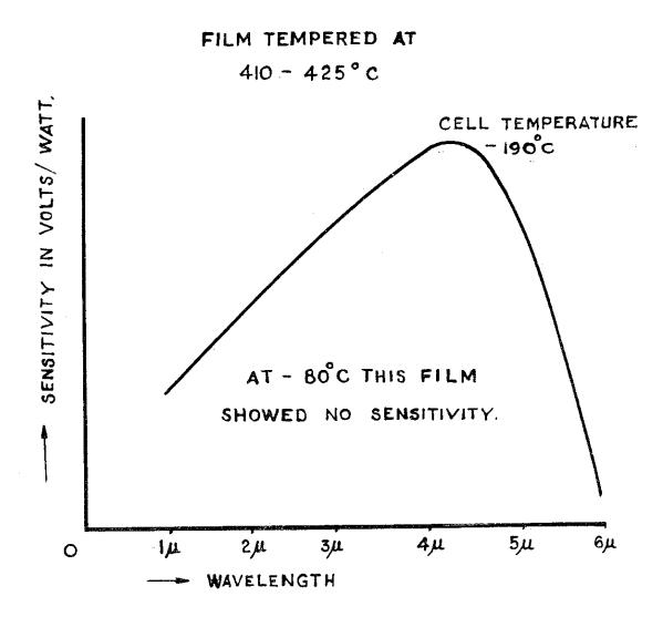
SPECTRAL SENSITIVITY CURVE FOR A LEAD TELLURIDE CELL. (1)
