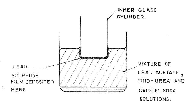
METHOD OF DEPOSITING LEAD SULPHIDE FILM.
